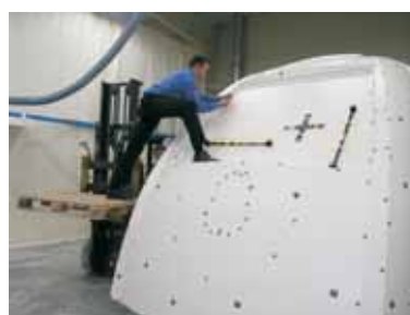
Measurement of a front FRP hood
